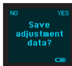
To save the adjustment, press either the Softkey for YES or the operating button.
