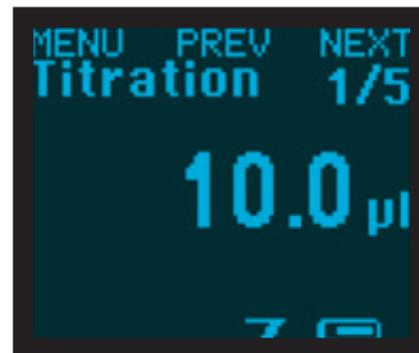
Titration has been programmed as the first step out of five.
