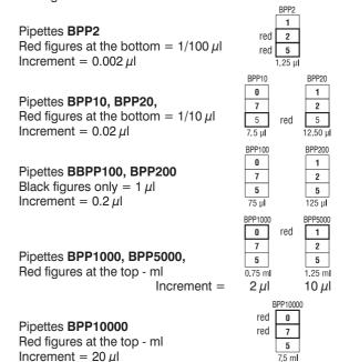
The volume of the pipette is set by the knob in the pipetting pushbutton (Fig. 1A2) or by the adjustment knob (Fig. 1B). The volume adjustment can be performed when the locking ring is set in the lower position (fig. 5A). When the desired volume is selected, the the locking ring should be set in the upper position (Fig.5B). To attain the maximum accuracy, set volume must be approached from a higher value by diminishing counter readings.
