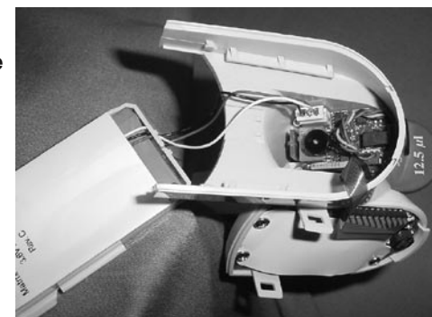
Figure F.3.2e: Remove Console Cover
