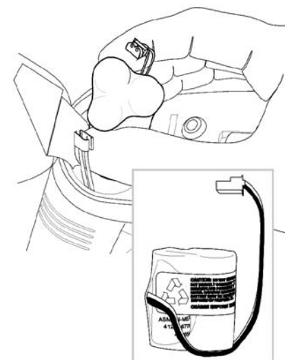
Figure F.3.1Ac: Remove Battery
