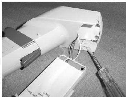
Figure F.3.2c: Unclip Snaps
