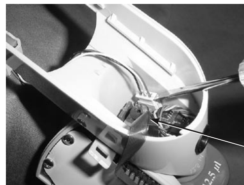
Figure F.3.2f: Lift Battery Connector
