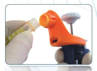
To close, return the tube to the secured cap, and rotate the tube until it is tight and remove.
