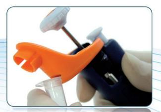
1 Insert the tab into the slot.
