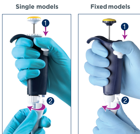
Figure 17 Removing the tip ejector.
