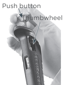
Figure 4 Location of Push Button and Thumbwheel
