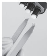
The use of tweezers to insert or remove a Safe-Cone Filter
