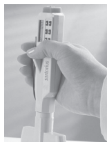
Squeeze the tip ejector lever, to eject the tip
