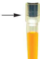
Visible seal when tip is loaded tightly
